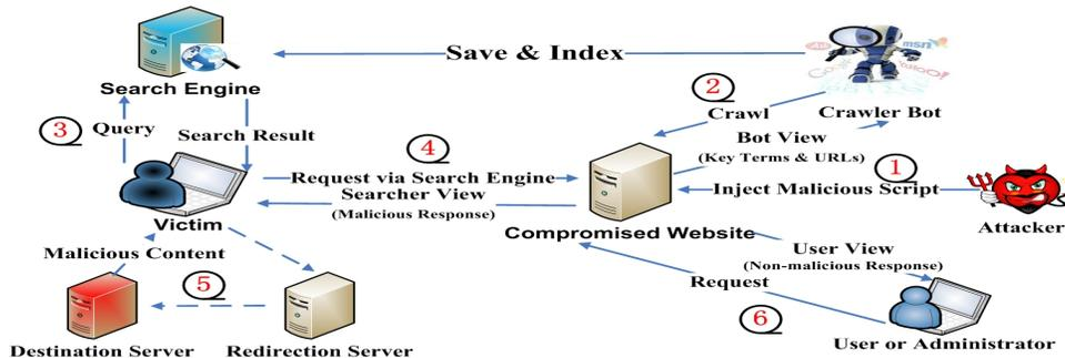
Fig. 1. The work flow of search poisoning attacks.
