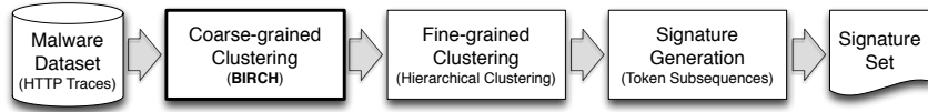
Figure 1: Overview of our new scalable behavioral malware clustering and network signature generation system.
